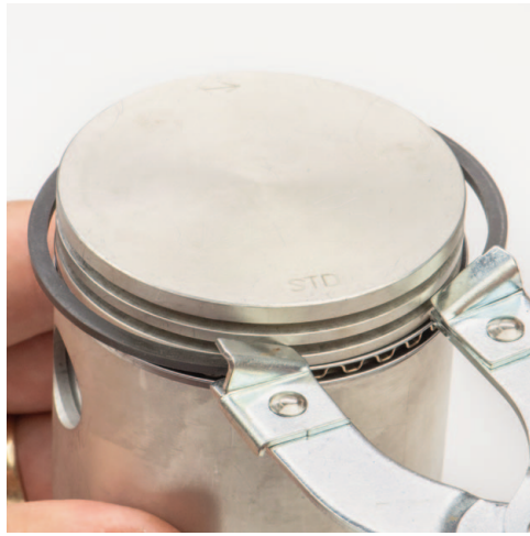
Using ring pliers gently expand the second ring over the piston and release into the second groove.
