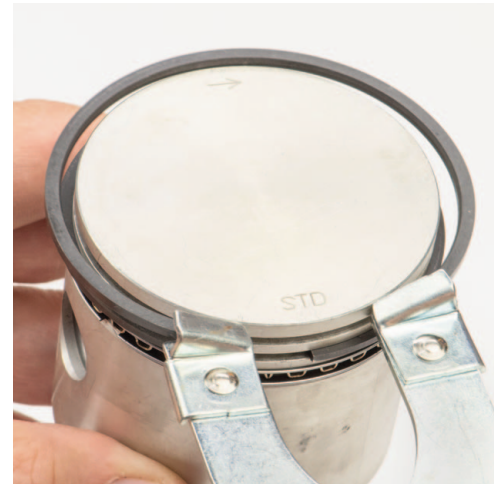
Using ring pliers gently expand the top ring over the piston and release into the top groove.
