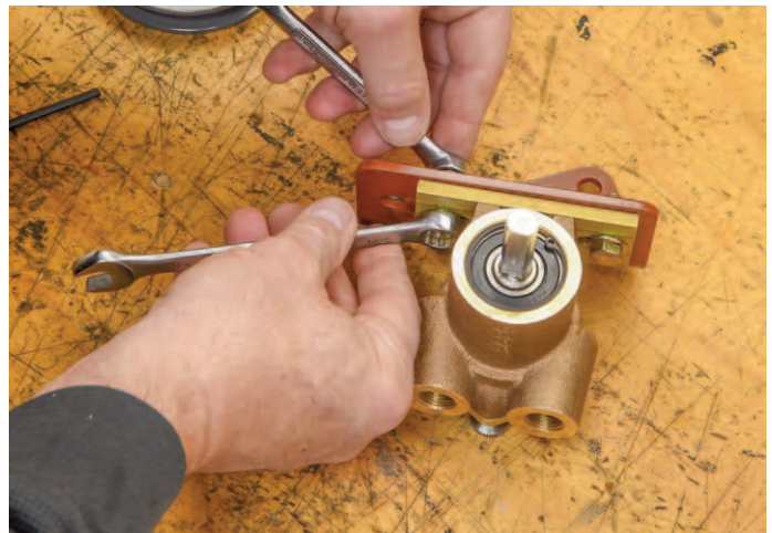
Mounting seawater pump to front mounted bracket
