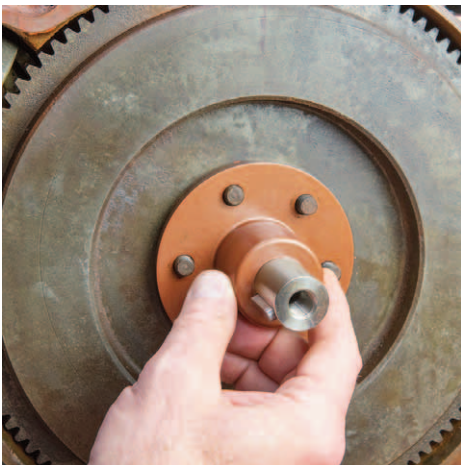
Install PTO shaft over flywheel studs (flywheel housing cover removed) (photo 1).
