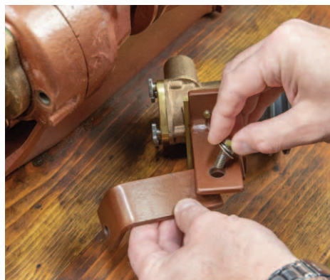
Remove right angle from pump bracket by removing pivot bolt (photo 5).
