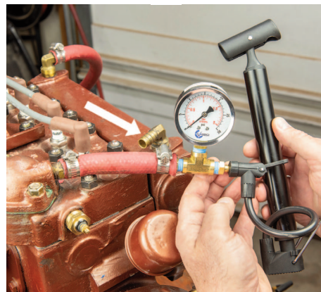
Cooling crossover hose disconnected from manifold hose barb (arrow), kit gauge assembly installed in hose, hand pump attached to Schrader valve, ready to pump.
