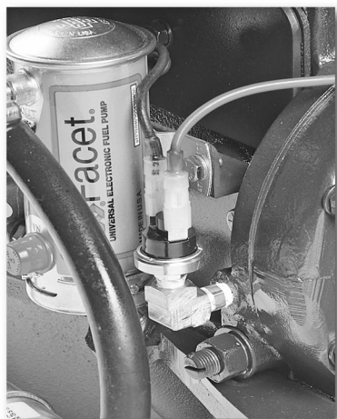
Factory installation, using 1/8" NPT oil port located above oil pressure regulating adjusting valve.
