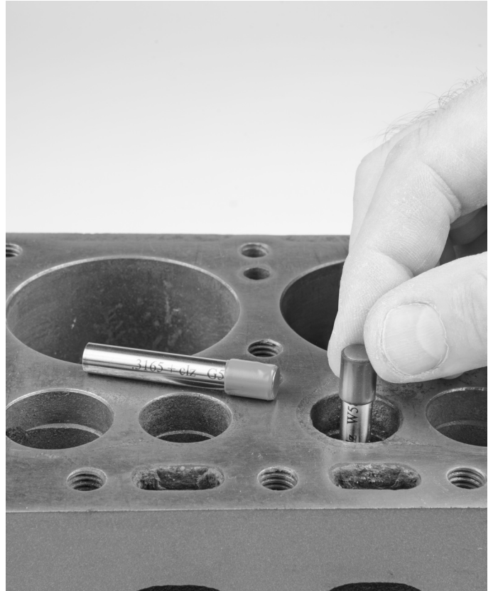
Measuring valve stem to valve guide clearance
