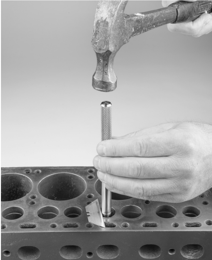
Installing new guide using depth mark
