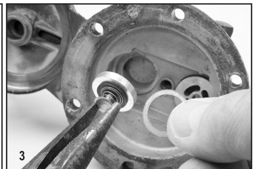
Close up of intake valve with gasket
