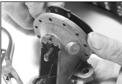
With link pin removed, the diaphragm is pulled out
