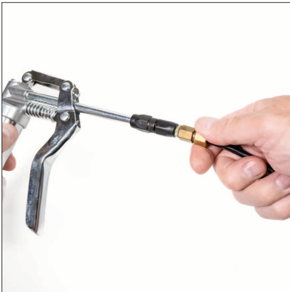
Push the grease fitting on the other end of the feed tube into your grease gun coupler (nozzle). You may tighten the locking nut on the coupler to lock the grease fitting in place when pumping if needed. Start pumping until grease fills the feed tube and squirts out the other end.
