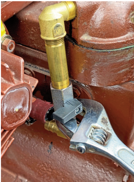
Fine tune hose barb angle to line up with hose
