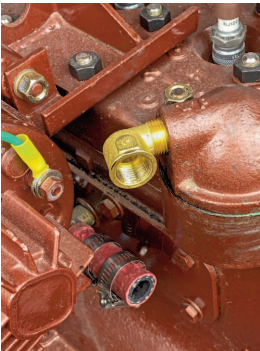
Street el facing flywheel end of engine
