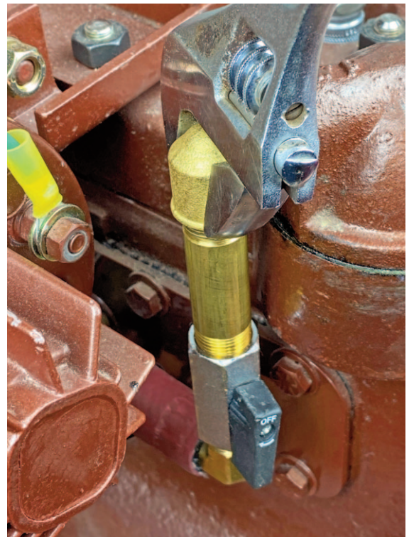
Turn fittings to fully seat hose barb in hose
