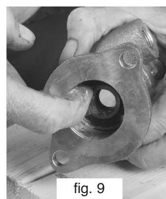
**NOTE:** Earlier models of MMI 502 flange pumps had the oil seal located at the flange end of the pump. Please pay close attention to reassembly step 6 and photo #12 and move the oil seal to the impeller side of the bearings. In this location, the seal will protect the bearings from water damage in case of a leaky water seal.
