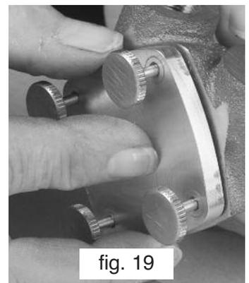
**NOTE:** The threads in the outside end of each of the thumb screw holes in the housing, have been drilled out to a depth of approximately 1/16" to accommodate the tips of the thumb screws. In this way, the ends of the thumb screws become "self-locating" when positioning the plate during installation. This feature makes it considerably easier to locate the back plate when replacing an impeller on the boat, where access is poor.
